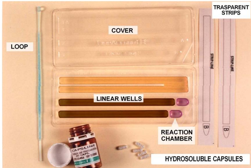
Fig. 1. Representation of the Linearcount 3MA system for *Campylobacter* isolation. The samples are cultured in the linear wells, which contained MacConkey agar, Skirrow and Karmali media; the CO<sub>2</sub> generating capsules are dissolved into the reaction chambers and the wells are sealed with the sealing strips; the wells are then protected with the transparent plastic cover and incubated at 37°C for 48 h in a normal-atmosphere incubator.
