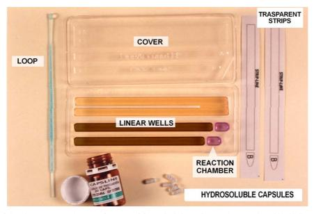
Fig. 1. Representation of the Linearcount 3MA system for *Campylobacter* isolation. The samples are cultured in the linear wells, which contained MacConkey agar, Skirrow and Karmali media; the  $CO_2$  generating capsules are dissolved into the reaction chambers and the wells are sealed with the sealing strips; the wells are then protected with the transparent plastic cover and incubated at 37°C for 48 h in a normal-atmosphere incubator.
